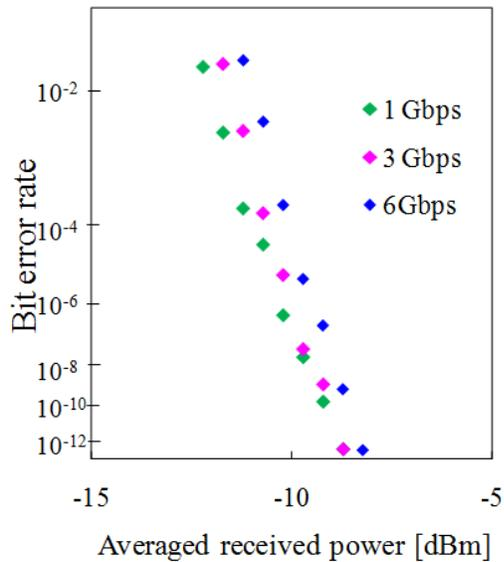
Fig. 8 BER measurements at 0V condition and eye patterns.
