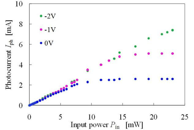
Fig. 4 Input light intensity dependence of photocurrent.
