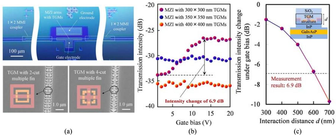
Fig. 2 (a) Plan-view optical microscope image of the permeability-controlled optical modulator (upper). Oblique view of TGMs for MZ arms, observed with SEM (lower). (b) Transmission characteristics of the device as a function of gate bias, measured for 1550-nm TE-polarized light. (c) Transmission intensity change of the device as a function of an interaction distance of the TGM, calculated by finite difference methods.
