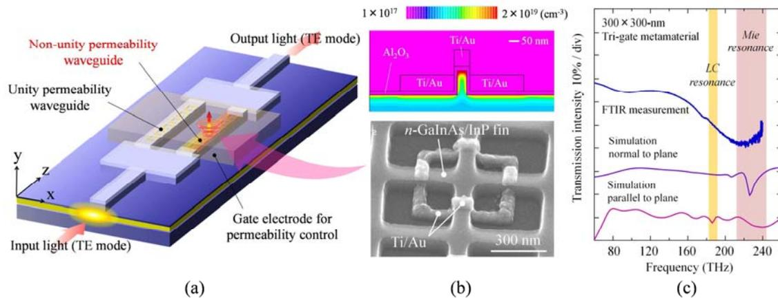
Fig. 1 (a) Permeability-controlled optical modulator consisting of InGaAsP/InP Mach-Zehnder interferometer with Tri-gate metamaterials. (b) SEM image of TGM unit cell (lower). Electron densities in the fin at  $V_g = 10$  V, calculated by 3-dimensional TCAD simulation (upper). (c) Normal-incidence transmittance spectra for  $300 \times 300$  nm TGM.
