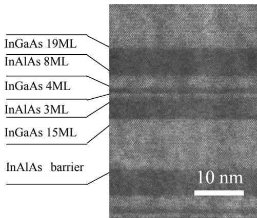
Fig.1. shows a transmission electron microscope (TEM) image of the cross-section of the FACQW wafer grown by MOVPE.
