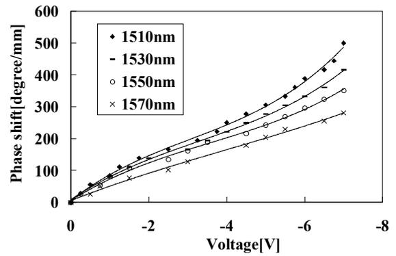
Fig.3. Phase modulation characteristics of the FACQW phase modulator.
