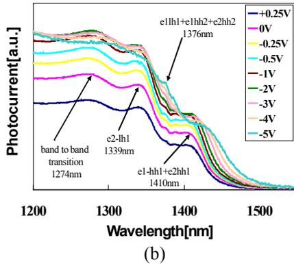
Fig.2. (a) . Calculated absorption spectra of the FACQW. (b) Measured photo-absorption current spectra at room temperature.
