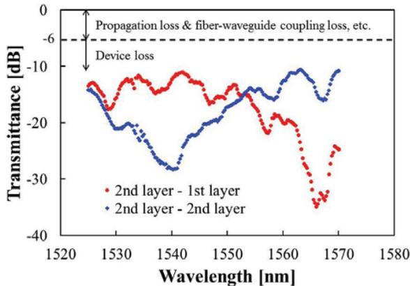
Fig.4 Measured transmitted power versus wavelength.
