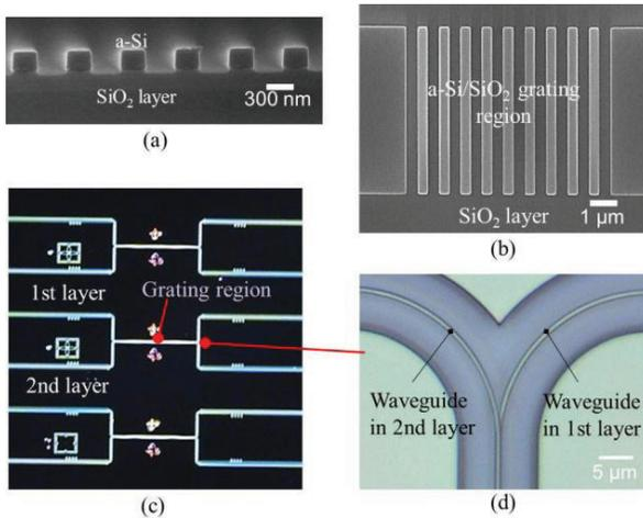
Fig.3 (a) Cross-sectional and (b) top SEM images of gratings (pitch : 640 nm, period : 10), optical microscope images of (c) a plan view of fabricated device and (d) enlarged Y branch.
