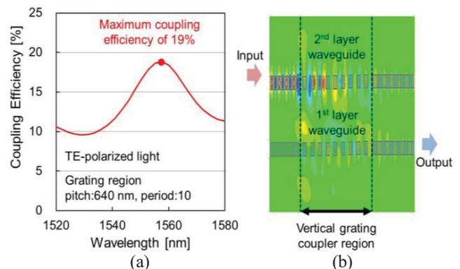
Fig.2 (a) Calculated coupling efficiency versus wavelength (b) the electric field distribution at grating coupler region.
