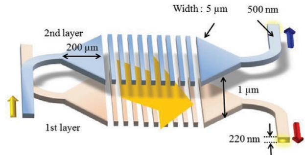
Fig.1 Device structure.
