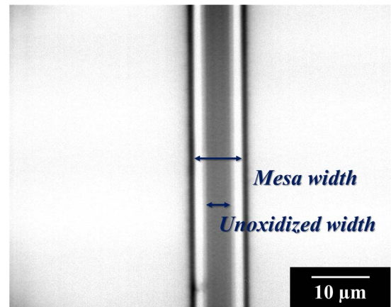
Fig. 2. IR microscopic top view of an oxidized mesa.
