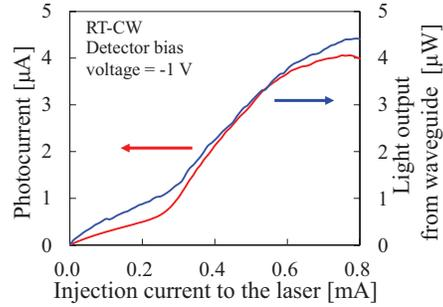
Fig.4 Photocurrent-injection current to laser characteristics.
