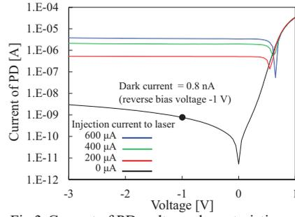
Fig.3 Current of PD-voltage characteristics of under various injection currents to the laser.
