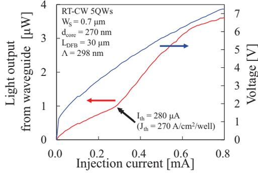
Fig. 2 Light output and voltage-current characteristics of  $\lambda/4$ -shifted membrane DFB laser.
