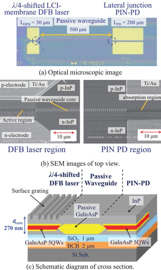
Fig. 1 Structure of the fabricated device.
