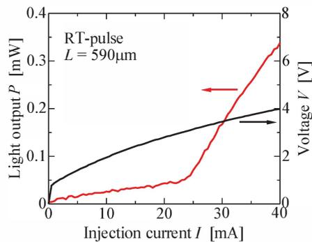
Fig.2 Lasing characteristics of the current injection-type membrane laser.
