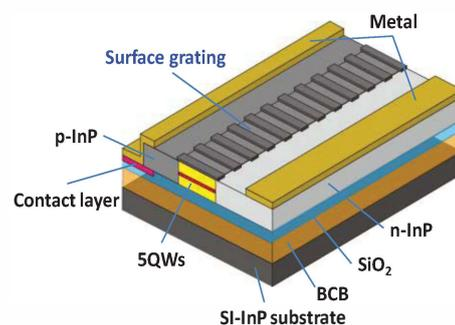
Fig. 1 Schematic device structure of LCI membrane DFB laser.
