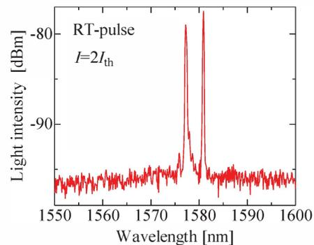
Fig.3 Lasing spectrum of the current injection-type membrane laser.
